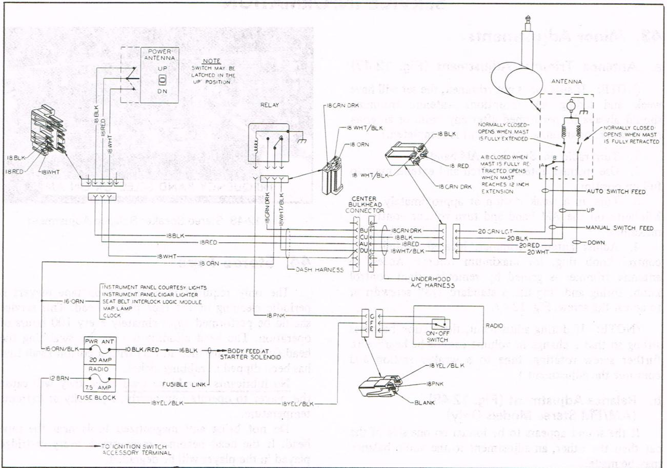
Fig. 12-46 Electric Antenna Wiring Circuit Diagram
