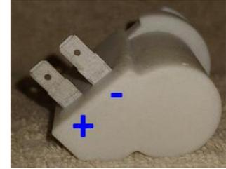
**Note 5: There is a polarity to the electrical connector. This MUST be maintained with the “+” terminal in the position shown. If you don't know which terminal is positive you MUST verify it else you may damage the new FIV.**
