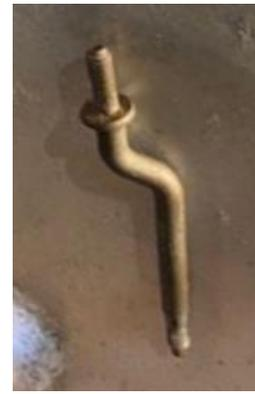
Note 4: The air cleaner lid rod will likely not be in the proper position fully threaded. Back-off until it is properly aligned. The wing nut will ensure tension on the rod and that's all that is required.
