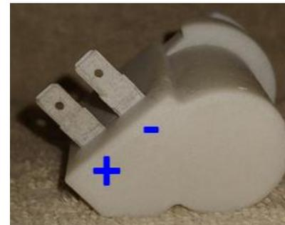
**Proper polarity of the electrical connector
