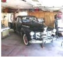
My work continues on my 41 Cadillac. The windshields have been installed, the wipers work, the dash has been reinstalled with a new glove box. It took several days to paint, color sand and polish the dash. My car now runs on a 12-volt system instead of the original 6-volt system. All the lights are much brighter so it should be much safer to drive after dark.
