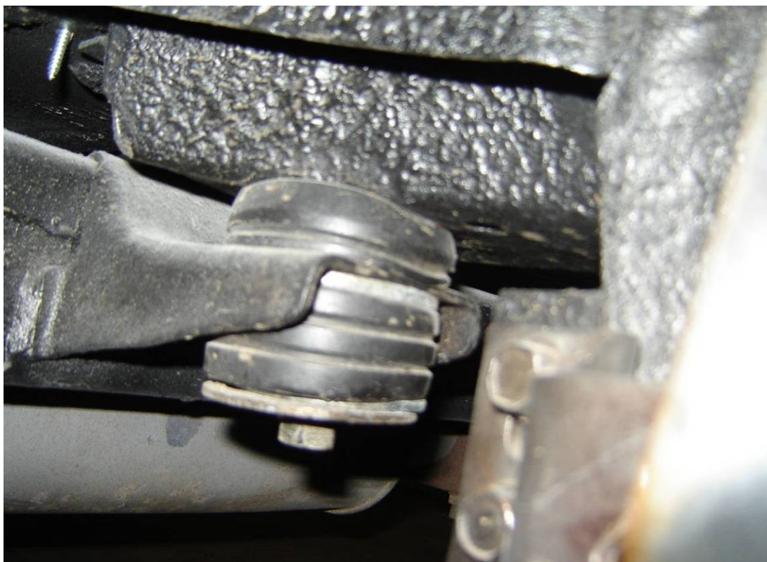
Mission accomplished: replaced bushing
