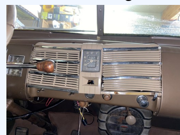
Radio/dash panel. Warped due to heat and age
