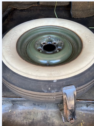
Original (?) spare tire with factory painted rim showing double pin-stripes
