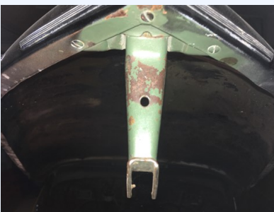
Hood latch, original factory color, the only part not painted black
