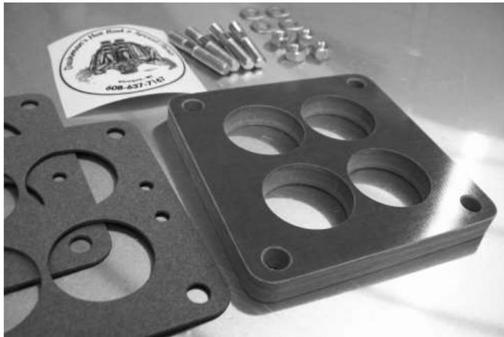
This 1/2" thick phenolic riser for the Small Carter WCFB 4 barrel carb that has the 3 7/8" x 3 3/4" stud pattern and will fit other models as well. Add a little performance to your machine the cheap way, and keep the heat away from the carburetor to solve the heat soak or carburetor boiling issues. Includes free gaskets, nuts, and washers. Please email us or call 608-637-7167 for any questions at Dashman's Hot Rod & Speed Parts.
