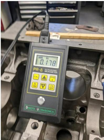
On this engine, maximum wall thickness:
