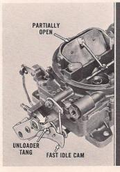
Choke Unloader: If the engine becomes flooded during a closed choke condition, a greater amount of air can be introduced into the intake manifold system by fully depressing the accelerator pedal. This action forces the unloader tang of the throttle lever against the fast idle cam and in turn partially opens the choke valve.
