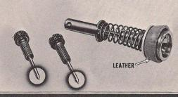
Inspect the tapered sections of the idle mixture screws for grooves or ridges. Replace if worn or threads are damaged. Inspect the pump plunger leather for cracks or creases. Replace with a new pump assembly if the leather is hardened, damaged, or shows signs of excessive wear.
