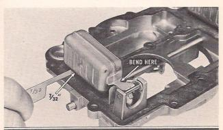
Float Level: Clearance between the air horn gasket surface and the top of the floats at their outer ends should be  $V_{32}$ ". Adjust by bending the float levers at the location shown. Recheck float alignment.
