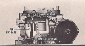
Hot Idle Compensator: This unit controls the opening and closing of a separate internal air passage in the carburetor main casting leading to the intake manifold. Throughout normal operating temperature ranges of the engine, the bimetal spring holds the valve tight to the seat.
