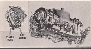
The heated air passes around the thermostatic coil spring and flows down the slotted sides of the piston bore before reaching the intake manifold vacuum source between the primary bores.
