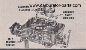
Remove the secondary venturi attaching screws, secondary venturi cluster assemblies and gaskets. Remove the auxiliary valve assembly by lifting straight upward. Remove idle mixture adjustment screws and springs.
