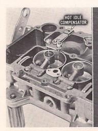
Remove the hot idle compensator and gasket. This unit is used on the rear carburetor of a 409 cubic inch engine equipped with TWO AFB carburetors and on both AFB models used on the 327 High Performance engines.
