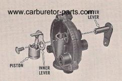
Remove the choke piston inner lever attaching screw. Separate the choke piston outer lever shaft from inner lever. Remove the choke piston and lever assembly.
