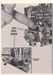
Choke Piston and Linkage: Connect the choke shaft clamp lever and rod. Insert the bent portion of a .026" wire gauge (part of J-9550 gauge set) in the top section of the slot cast into the choke piston bore. Slowly rotate the choke inner piston lever clockwise until the gauge is held tightly in the top of the slot by the piston. Hold this position and proceed as follows.
