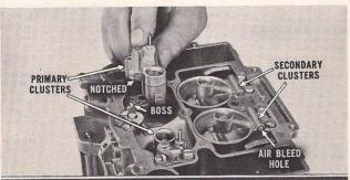
Install the primary and secondary venturi clusters with new gaskets. The primary clusters are notched to align with the boss in the casting. The secondary clusters are correctly installed with the air bleed holes (horizontal bronze housings) pointing toward the outside of the casting. Tighten attaching screws securely.
