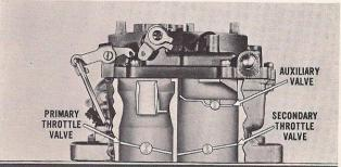
Throttle and Auxiliary Valves: Fuel and air flow of all AFB carburetors is controlled by the primary and secondary throttle valves and the auxiliary valves. The primary throttle valves function at all engine speeds regardless of the choke valve position. The secondary throttle valves function only with a wide open choke in the following manner.
