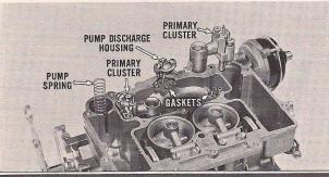
Remove the accelerator pump spring. Remove the primary venturi attaching screws, primary venturi cluster assemblies and gaskets. Remove the accelerator pump discharge housing attaching screws, housing and gasket.
