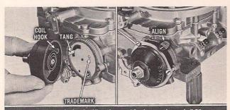
Install the choke baffle plate with the trademark "C" facing outward and place the gasket in position. Install the choke cover so that the coil hook engages with the tang on the choke piston inner lever. Loosely install retainer with screws. Then, rotate the cover clockwise to align the index mark with the middle mark on the housing and tighten screws.
