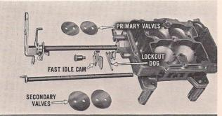
Remove the fast idle cam and lockout dog. File the peened ends of the throttle valve attaching screws; then remove the screws. Remove the primary and secondary throttle valves. Check throttle shafts for burrs at screw holes. Smooth off any roughness; then remove shafts.
