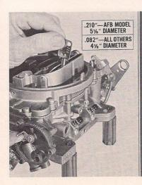
Measure the distance between the top of the choke valve and the air horn wall as shown. The choke opening should be .210" for the AFB model with a 5½" diameter air horn throat and .082" for all others with a 4½" diameter air horn throat.
