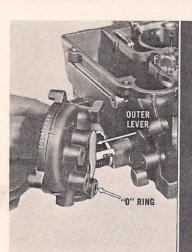
Install the choke piston outer lever in the choke housing. Insert the choke piston in the bore and attach the piston inner lever to the outer lever with the screw. Position a new "O" ring seal in the housing and attach the unit to the casting with the three screws.
