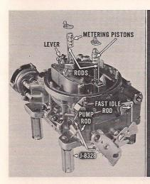
Support the carburetor on a suitable fixture or legs such as J-8328 to protect the throttle valves and linkage from damage. Remove the cover screws and plates holding the metering pistons, rods and springs to the air horn. Disconnect the upper end of the fast idle rod, the choke shaft clamp lever and the lower end of the accelerator pump rod.
