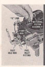
Install the pump "S" link, pump arm and the attaching screw. Install the pump rod to the pump arm and throttle lever with the spring clip and snap retainer. Connect the fast idle rod and install the spring clip. Install fuel inlet fitting with a new gasket. Install metering piston assemblies.
