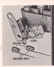
Check the steps on the fast idle cam for excessive wear and all movable linkage parts for an out-ofround condition or enlargement of the pivoting holes. Inspect vacuumoperated pistons and metering rods for damage. Replace parts as necessary to insure proper operation of the carburetor.
