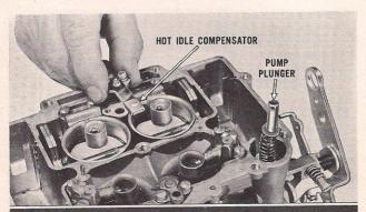
If the carburetor is equipped with a hot idle compensator, install this unit with a new gasket at this time. Install the accelerator pump spring and pump plunger.
