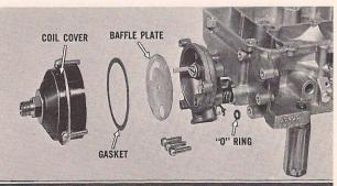
Remove the three screws attaching the choke thermostatic coil cover to the choke housing. Remove the gasket and baffle plate. Remove the choke housing attaching screws and separate the housing from the casting. Remove the small "O" ring seal.
