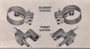
Carefully inspect the primary and secondary venturi clusters. Make sure there is no lint or foreign material obstructing the openings. If any of the preassembled parts are loose, bent or damaged, replace with a new cluster assembly.
