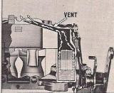
Fuel Bowl Vents: The vents perform two functions. They admit atmospheric pressure into the fuel bowls for proper carburetor operation. Also, when the engine is stopped and underhood temperatures greatly increase, fuel in the float bowls has a tendency to boil. The resulting fuel vapors escape through the vents rather than create a carburetor flooding condition.
