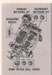
Remove the pump intake ball check assembly from the area adjacent to the accelerator pump cylinder. Remove the primary and secondary metering jets. Turn the casting upside down to remove the pump discharge needle. NOTE: The primary jets have larger holes to accommodate the metering rods.
