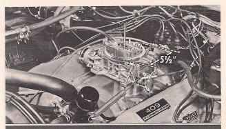
The 1962 Chevrolet passenger cars with the 409 cubic inch engine use Carter model AFB 3345SA, Chevrolet part number 3820580, as standard equipment. The air horn throat diameter is 5½ inches.
