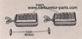
Shake floats to determine if fuel has leaked inside. Replace if necessary. Visually inspect float needles for signs of defects. Any history of leakage between the needle and seat, causing a flooding condition, should be corrected with new matched needle and seat assemblies.
