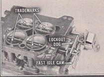
bores. Tighten the screws securely. Lightly upset screw ends to prevent them from falling out. Install fast idle cam and lockout dog. This completes throttle valve and linkage overhaul.
