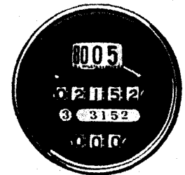
Figure 19. The lubrication notice is a continual reminder of when the next lubrication is due.
