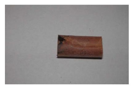
My plan is to replace the old aluminum foil type with a newer capacitor, now .3mf may be hard to find today the closes one would be .33nf (or 330000pf). This one is rated at 400V
