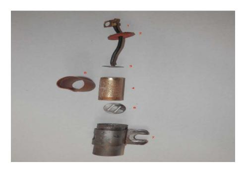
Everything 3, 4 and 6 is pressed tight inside forcing 6 to keep contact at the bottom for the ground path.
