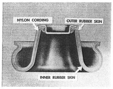
The bellows is composed of three layers — an outer rubber skin, a layer of nylon cording, and an inner rubber skin. The outer rubber skin is merely a protective cover — much like the paint on the body of the car, or the outer rubber casing on automobile tires. The strength of the bellows is in the nylon cording. The inner rubber skin prevents air from leaking out. Keeping this in mind, we can see why the only scorings we have to worry about . . .
