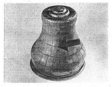
If the slit is vertical or horizontal, it is not running parallel to the cording, and -- as long as the slit is not deep enough to reveal the nylon cording -- the bellows should not be replaced.
