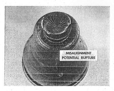
If the bellows is not properly aligned, it will not sit squarely on the piston, and the bellows may become kinked and eventually rupture. On the illustration to the left, you can see where the bellows was mispositioned on the piston.
