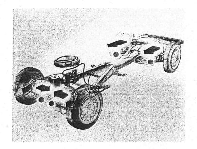
Also, the air domes should be positioned directly over the pistons. If they are not, an excess load on the suspension bushings will result.
