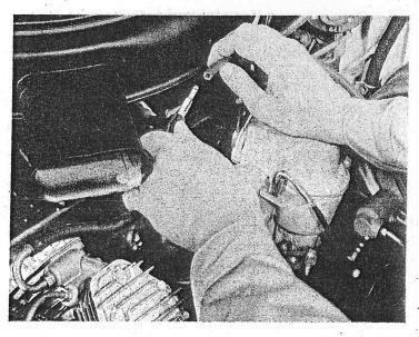
The correct amount of vapor will enter the system if we first purge the air from the accumulator tank, and then charge the accumulator tank with Freon-12 vapor, using the special adapter that will fit the accumulator service valve, Tool Number J-8731. We should charge the system until it reaches drum pressure, at which point you can no longer hear the hissing sound of the Freon vapor entering the accumulator tank. Disconnect the Freon drum.
