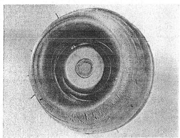
Cracks like this -- called ozone cracks -- are also all right, as long as they do not reveal the nylon cording. You've probably seen cracks like this on the side wall of tires. Just as tires are not weakened by these cracks, neither are the bellows. Ozone, by the way, is a form of oxygen, and is formed by a discharge of electricity in the air. It's also important to check the bellows for correct alignment and positioning.
