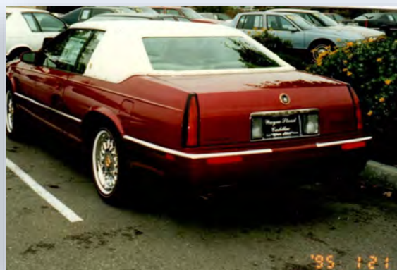
New 1995 Eldorado sim. Carriage top. Vogue "H" Tyres are safely performance-speed rated to 149 mph. Zero distortion. 1988 new FWD Cadillacs had 85 mph (max) speedometers and thin side wall tires.
