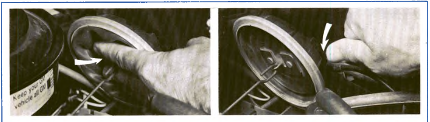
Figure 1-18b, Cover Vacuum Port and Release Finger Pressure on Diaphragm.
