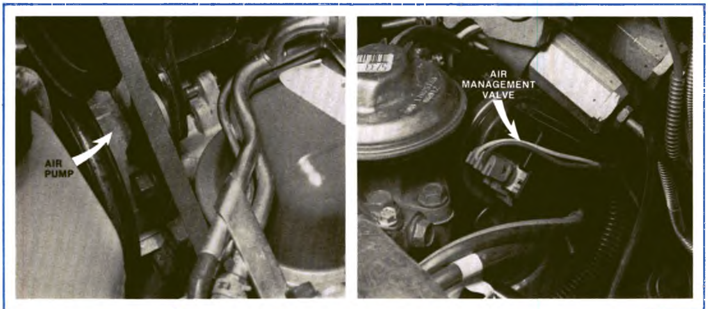
Figure 3-1, Typical Air Pump, and Air Management Valve Installation.
