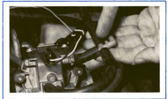
Figure 1-17, Physical Inspection of the Vacuum System.
