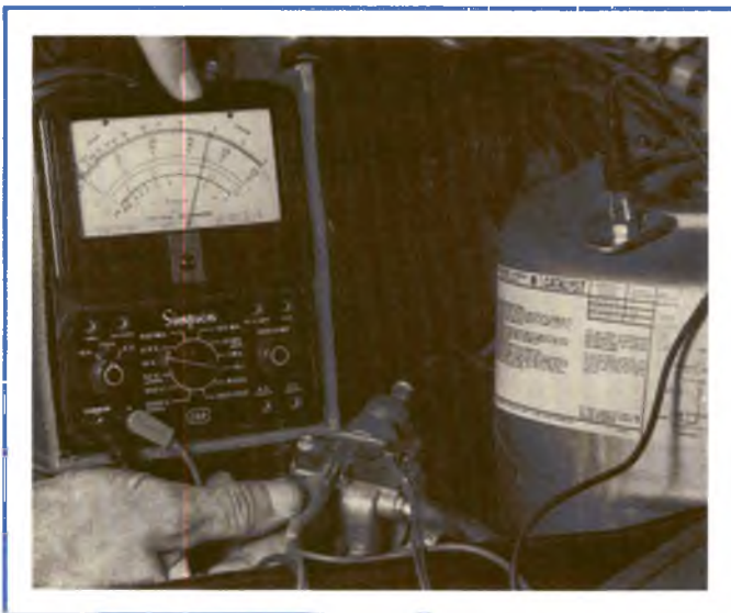
Figure 2-8, Check Resistor Wire and Transducer Solenoid Coil with an Ohmmeter.
