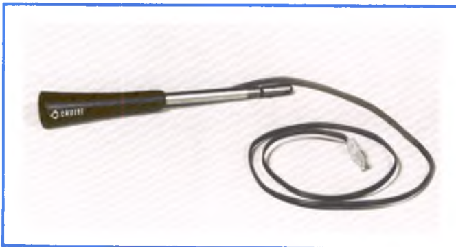
Figure 1-5, Cruise Control Lever with Engage Switch Button.
