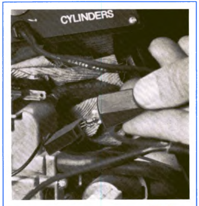
Figure 2-6, Check Resume Solenoid Valve Connector with Voltmeter.
