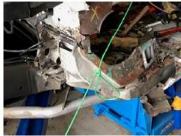
Cutting out the A pillar
