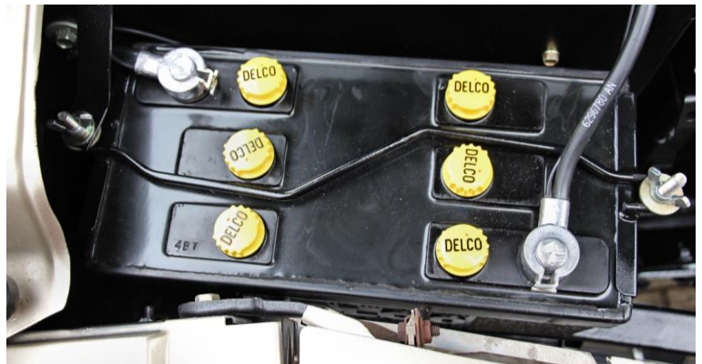
Picture Above: Note from picture of Jim Verraster's featured Cadillac, that the 1963 has a piece that goes from radiator support across to bracket on upper grill support bar which is unlike the side-to-side hold down on the 1964 Cadillac.
