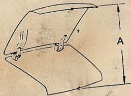
RAISE LID TO FULL EXTENSION OF GAS SUPPORTS. PROP LID IN THIS POSITION AND MEASURE DIMENSION "A" BEFORE REMOVAL OF EXISTING GAS SUPPORTS.
