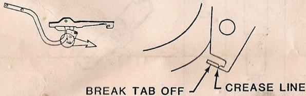
INSTALL #4 LOWER BRACKET TO #3 SUPPORT USING #7 NUTS. AND INSTALL SUPPORT ON HINGE ARM STUD.
